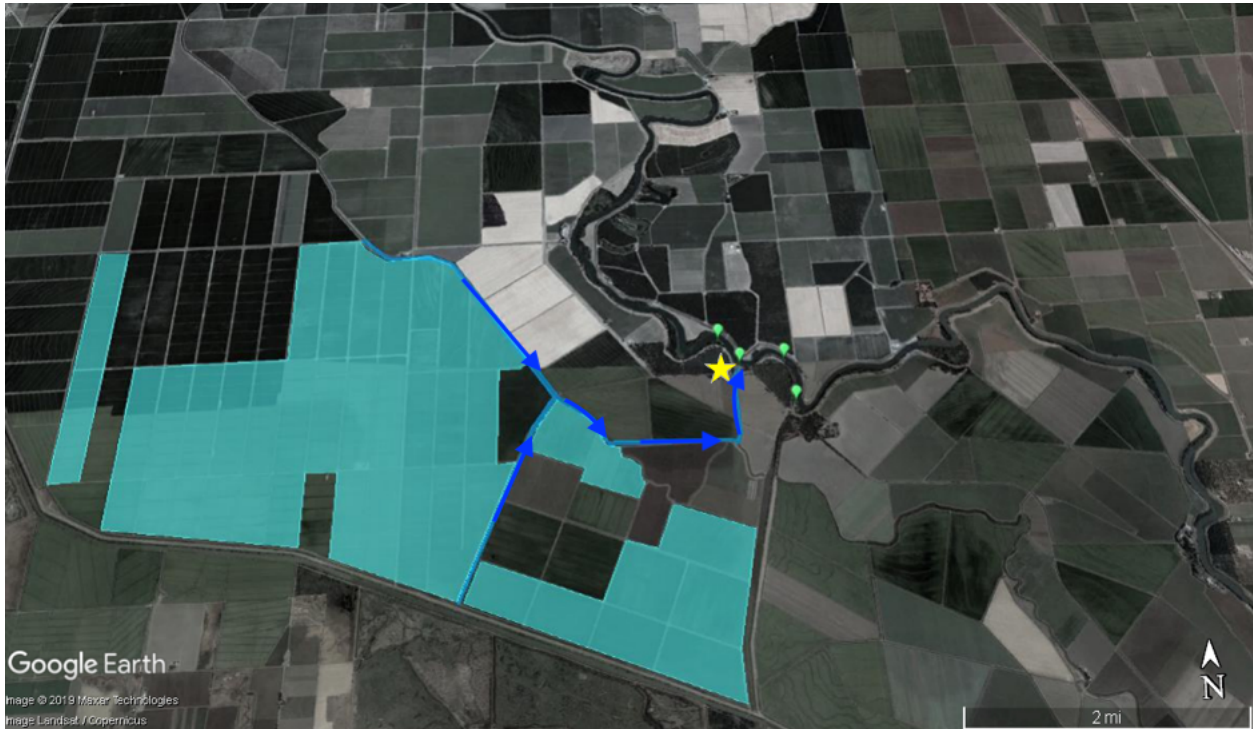
Figure 1: Study location in western Sacramento Valley just north of Knights Landing; The 5,435 acres of Reclamation District 108 and River Garden Farms fields inundated and drained as part of the experiment are shaded in blue, water drains via gravity from fields through canals shown with blue arrows to the Rough and Ready pumping station (yellow star) where it is pumped into the Sacramento River (flowing from north to south). Sample locations within the river where juvenile Chinook salmon were caged are shown with a green pin.
